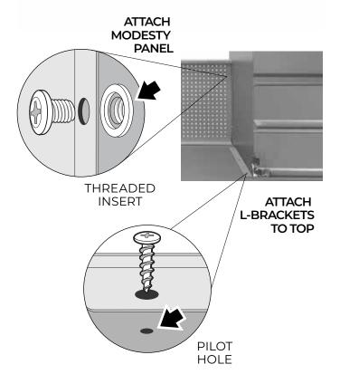
Attach the **Modesty Panel** to the Drawer Units using four (4) M6 truss head screws for each side.
