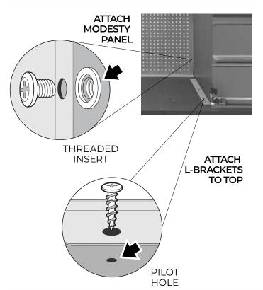
Attach the **M-Panel** to the drawer unit using two (2) M6 truss head screws.
